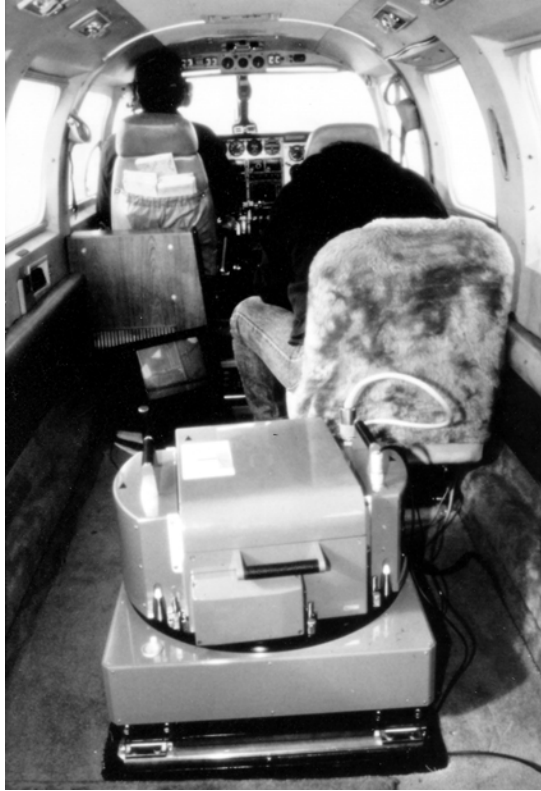
Figure 4.2 Typical aerial photographic installation. (Courtesy of Surdex Corporation, Chesterfield, MO.)
