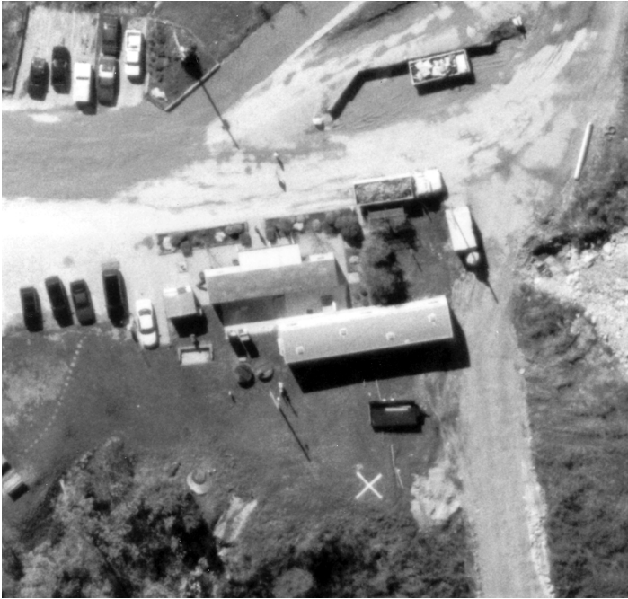
Figure 10.6 Ground target on an aerial photograph. (Courtesy of U.S. Army Corps of Engineers, St. Louis District.)
